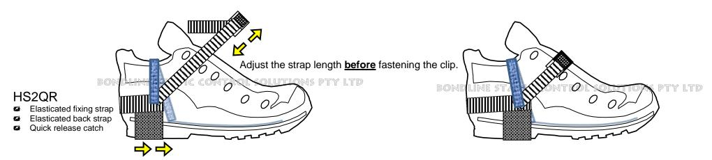
Pull against the elastic back strap, until the conductive strip is towards the front of the heel, to ensure a snug fit and help prolong strap life.
